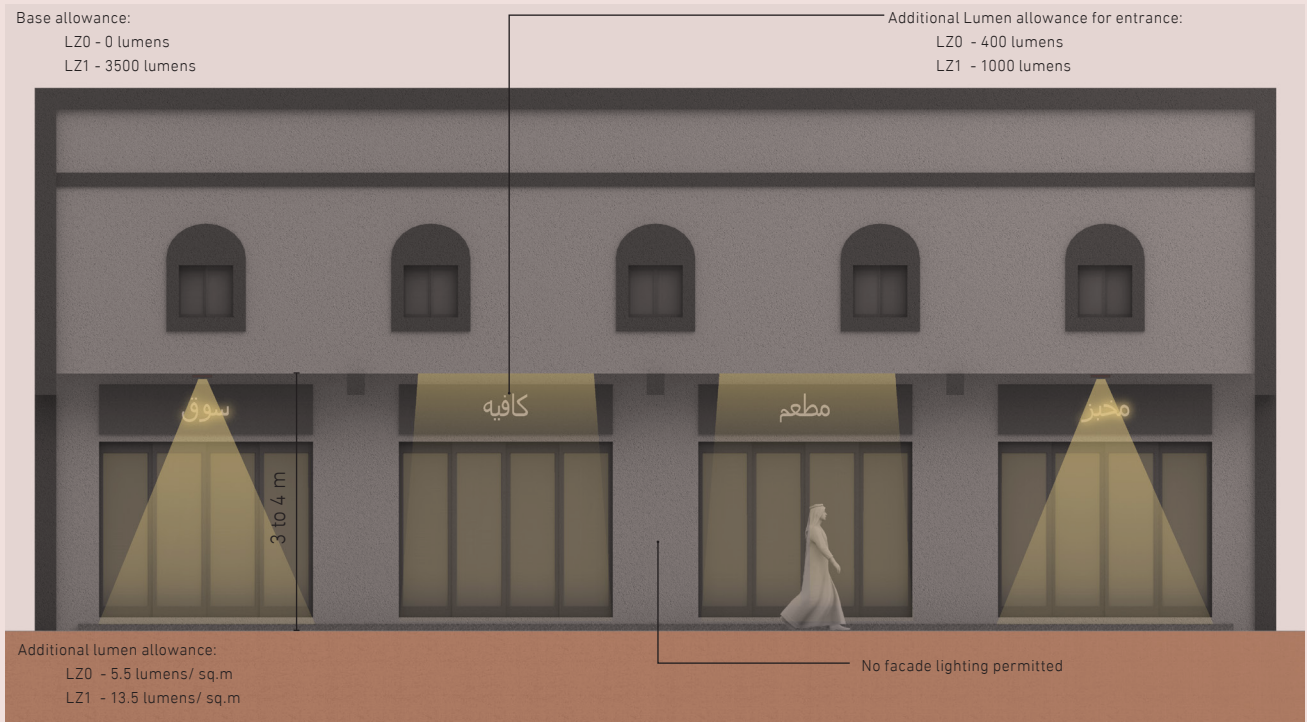
Figure 19: Lighting for commercial buildings in LZ0 & LZ1
