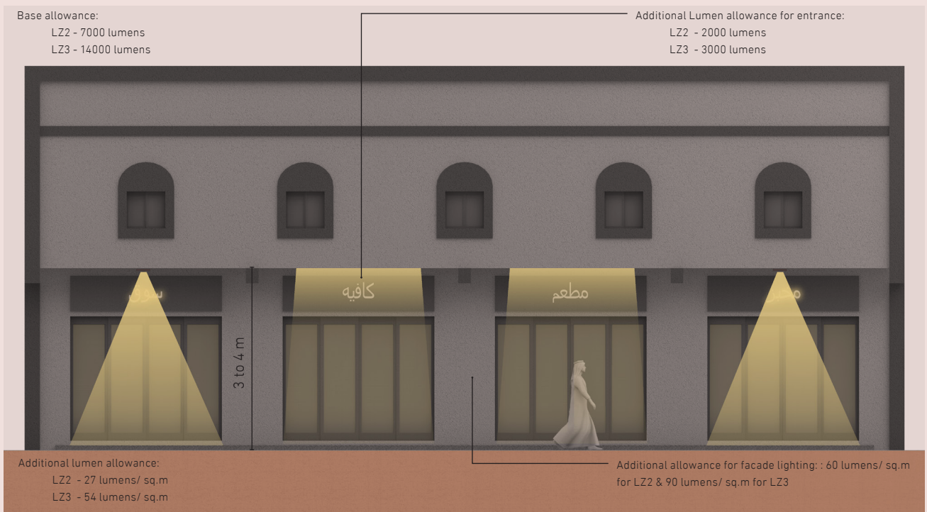
Figure 20: Lighting for commercial buildings in LZ2 & LZ3
