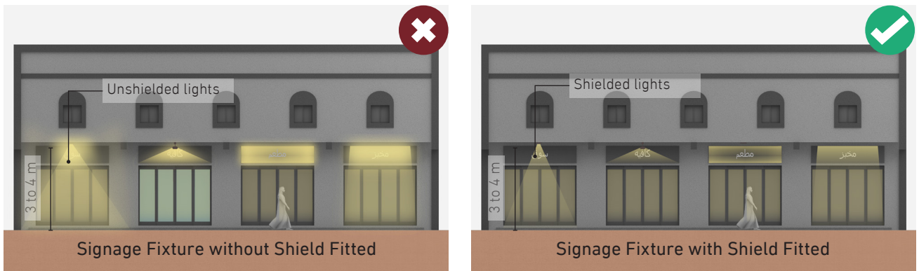
Figure 10: Retail Buildings shall align to lighting glare requirements for all facade fixtures and signage lights.
